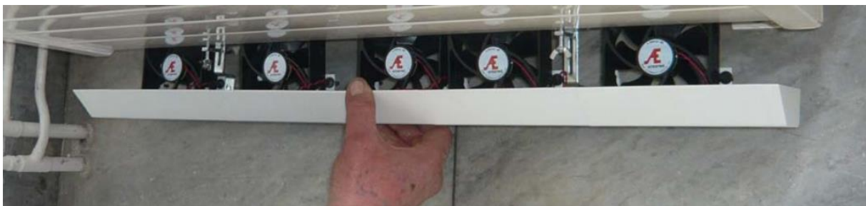
Figure 1.11: Five fans mounted on the cover [19]
