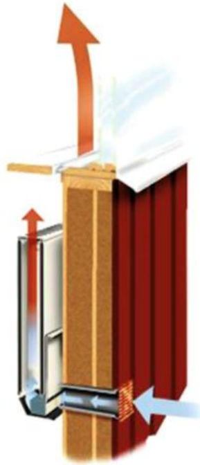
Figure 1.10: Built-up of a ventilation radiator [21]
