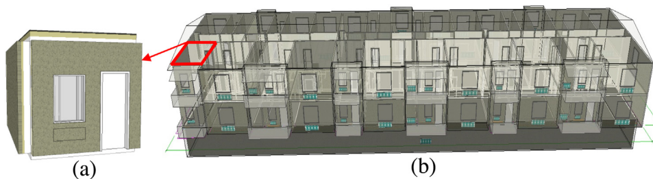
Fig. 4. Constructed building model in IDA ICE (Fig. 3b) and selected reference zone with the highest heating demand ((a), framed in red in (b)). (For interpretation of the references to color in this figure legend, the reader is referred to the web version of this article.)
