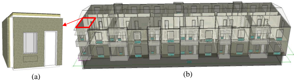
Figure 3. Constructed building model in IDA ICE (Fig.3b) and selected reference zone with the worst thermal performance (Fig.3a, framed in red in Fig 3b)
